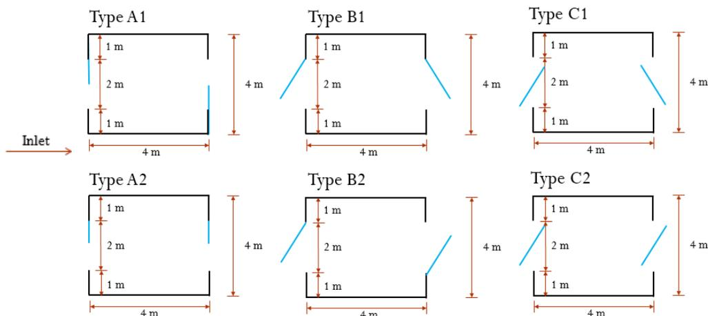
Figure 5: Top view for different types of windows. Type A shows horizontal slide window, Type B shows vertical turn window, and Type C shows vertical pivot window.
