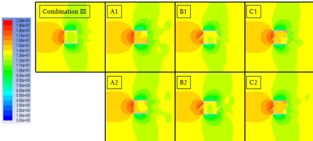
**Figure 8:** CFD results for three types windows: pressure (pascal).
