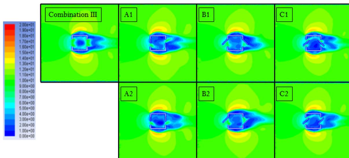
**Figure 9:** CFD results for three types windows: velocity (m/s).
