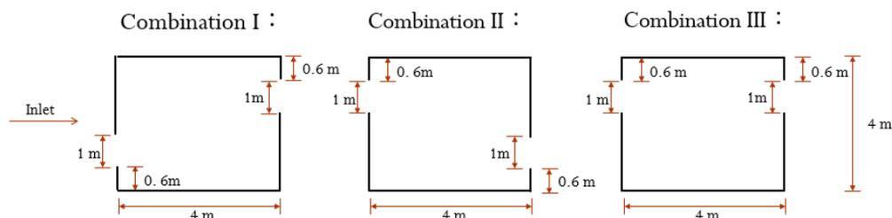
Figure 4: Side view for different combinations of windows.
