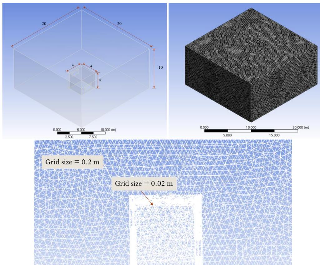
**Figure 3:** Perspective view with dimensions.
