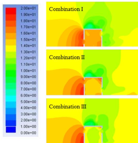
**Figure 6:** CFD results for three different combinations: pressure (pascal).
