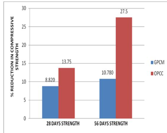
**Fig. 4.** Strength reduction due to Na<sub>2</sub>SO<sub>4</sub> attack on GPCM and OPCC
