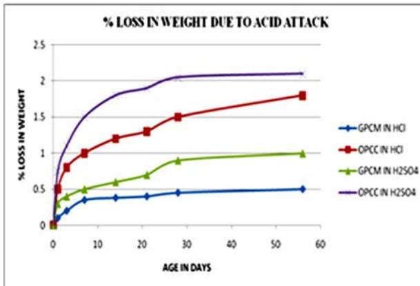
**Fig. 1** Acid attack on GPCM and OPCC
