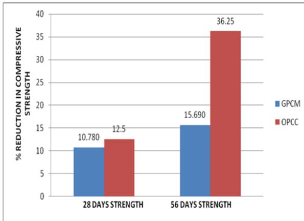
**Fig. 5.** Strength reduction due to NaCl attack on GPCM and OPCC
