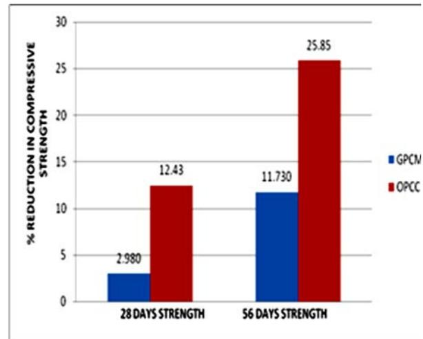
**Fig. 3.** Percentage of Strength reduction due to H<sub>2</sub>SO<sub>4</sub> Acid attack on GPCM & OPCC
