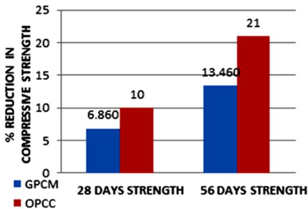
**Fig. 2.** Percentage of Strength reduction due to HCl Acid attack on GPCM and OPCC
