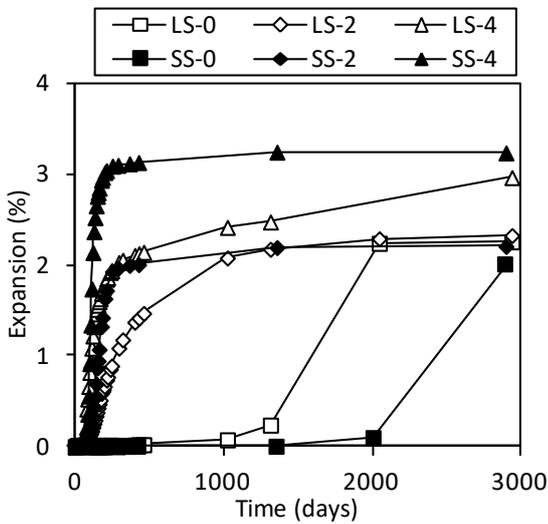
**Fig. 12.** Expansion behaviors of mortar using different type of aggregate (SS: Siliceous sand, LS: Limestone, Legend indicates “Aggregate type” - “SO<sub>3</sub> dosage”) (Kawabata *et al.*, 2015)
