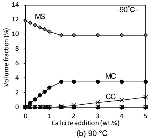
**Fig. 14.** Change in phase assemblage with increasing amount of calcite added in the system (W/C=0.50, CC: Calcite, MS: Monosulfoaluminate, MC: Monocarboaluminate, HC: Hemicarboaluminate, Ett: Ettringite)
