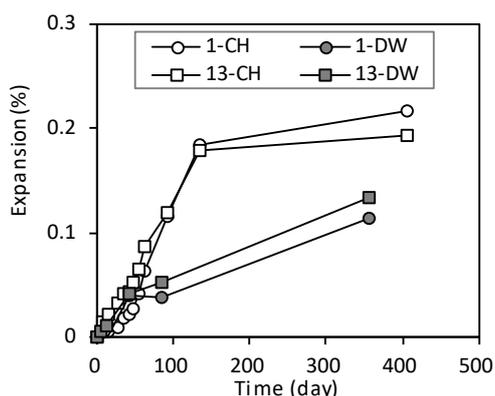
(b) 1 mol/l NaOH solution at 80 °C
