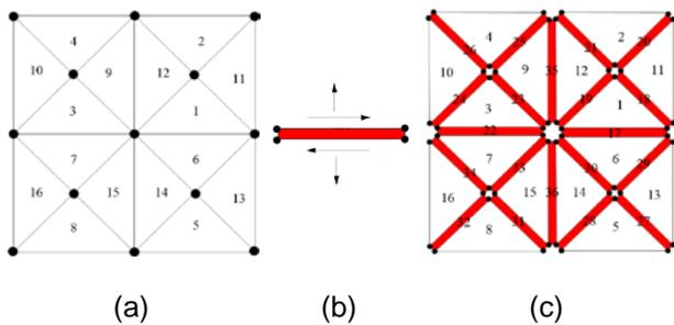
**Fig. 2.** Insertion process of cohesive elements: (a) initial mesh; (b) inserted cohesive element based on newly created nodes; and (c) mesh after insertion of cohesive elements
