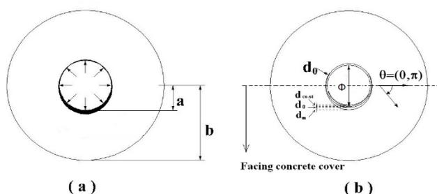
Fig. 1. Semi-elliptical corrosion model
