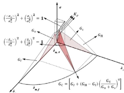
**Fig. 4.** Mixed mode fracture constitutive model
