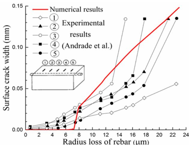
**Fig. 9.** Experimental verification of the crack width
