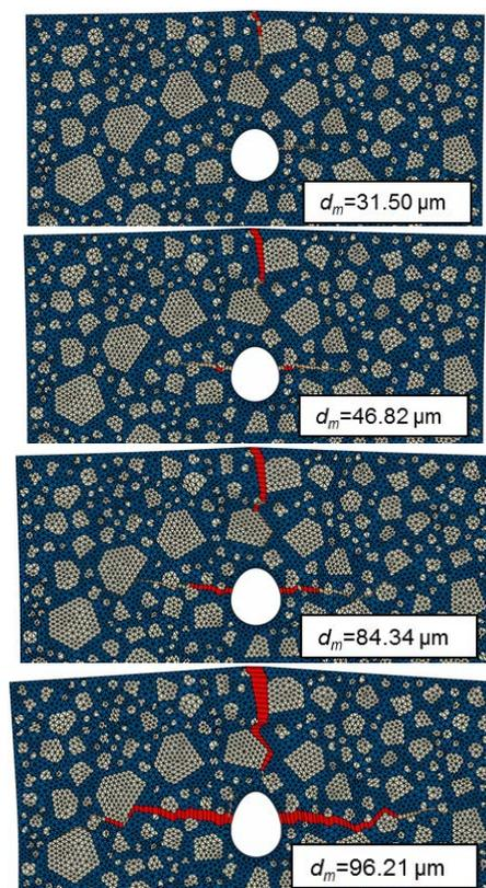
**Fig. 6.** Crack propagation of concrete induced by non-uniform corrosion of reinforcement
