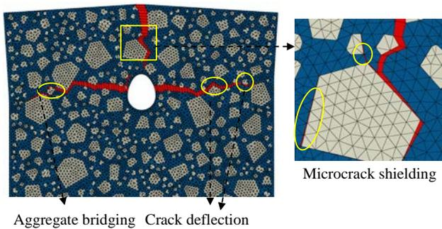
**Fig. 7.** Some toughening mechanisms in crack propagation process
