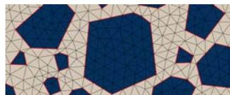
Interfacial cohesive elements between aggregates and mortar
