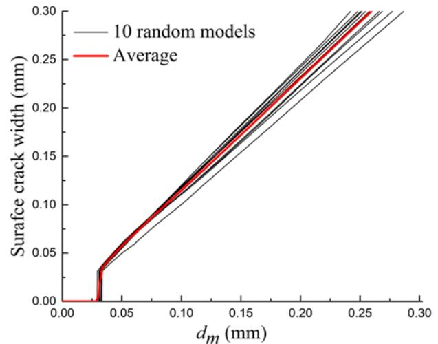
**Fig. 8.** Surface crack width as a function of corrosion expansion displacement for 10 meso scale models
