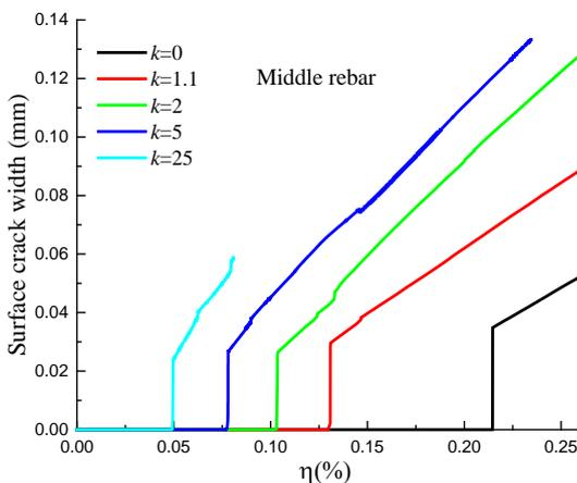
**Fig. 7.** Surface crack width induced by corrosion of middle rebar as a function of corrosion degree  $\eta$  under different non-uniform corrosion coefficient  $k$
