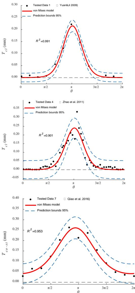
**Fig. 2.** Regression analysis of the developed von Mises model with test data
