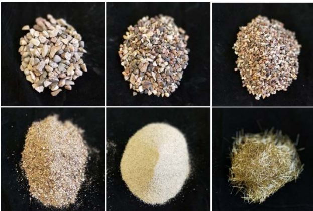
Fig. 2. Coarse aggregates (6.25mm, 4.75mm and 2.36mm), fine aggregates (coarse sand, fine sand) and steel fibers used in the study.
