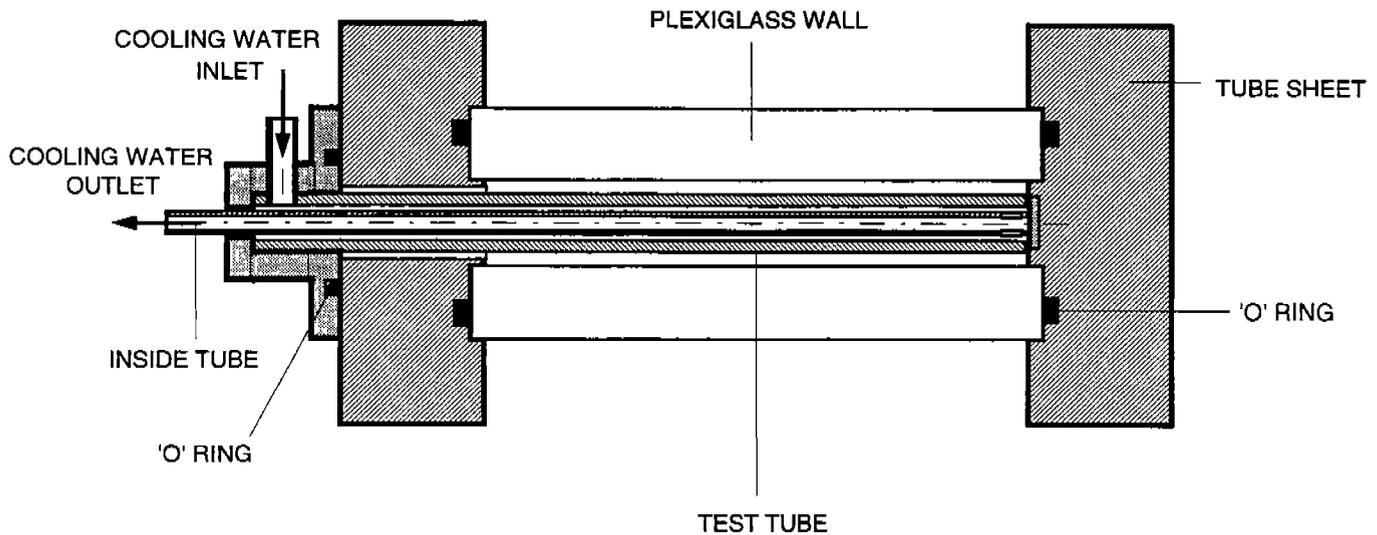
Fig.1 Experimental test section with transparent walls.
