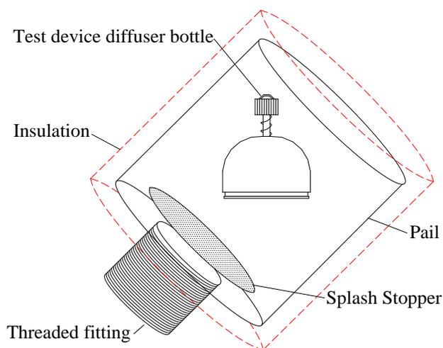
**Figure 3:** Test chamber design
