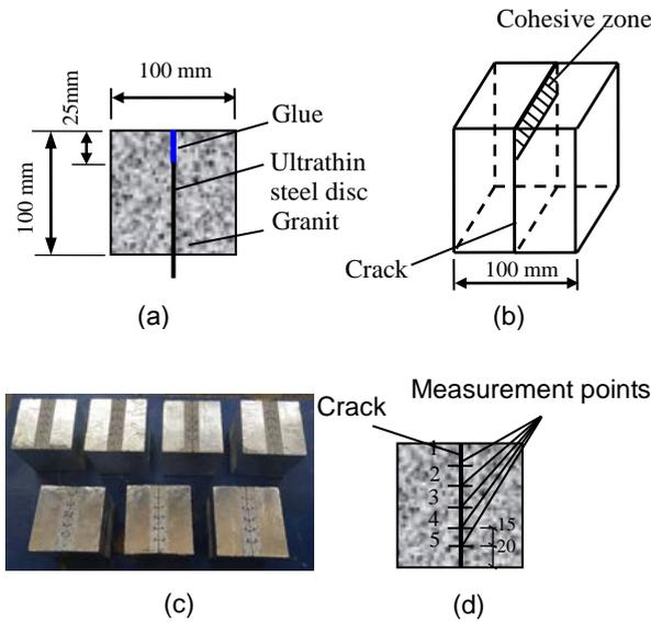
**Fig. 1.** Preparation of cracked specimens (a) front view of specimen fabricating; (b) specimen with a single parallel crack; (c) test specimens unsealed by epoxy; (d) measurement points for the bottom surface of a crack.
