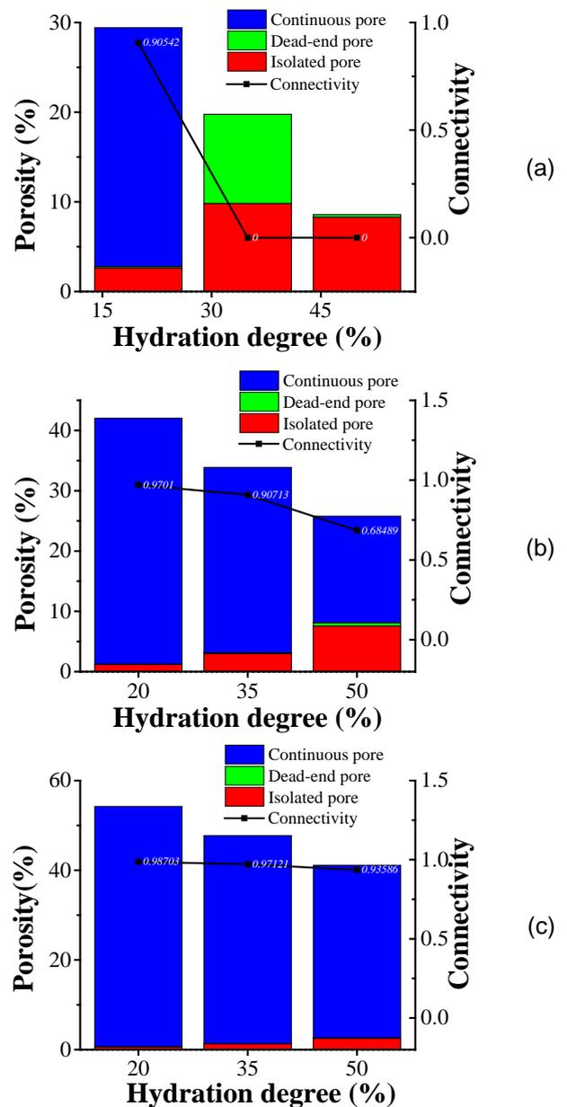
**Fig. 4.** The porosity of various types of pores in the three water - cement ratio of microstructure
