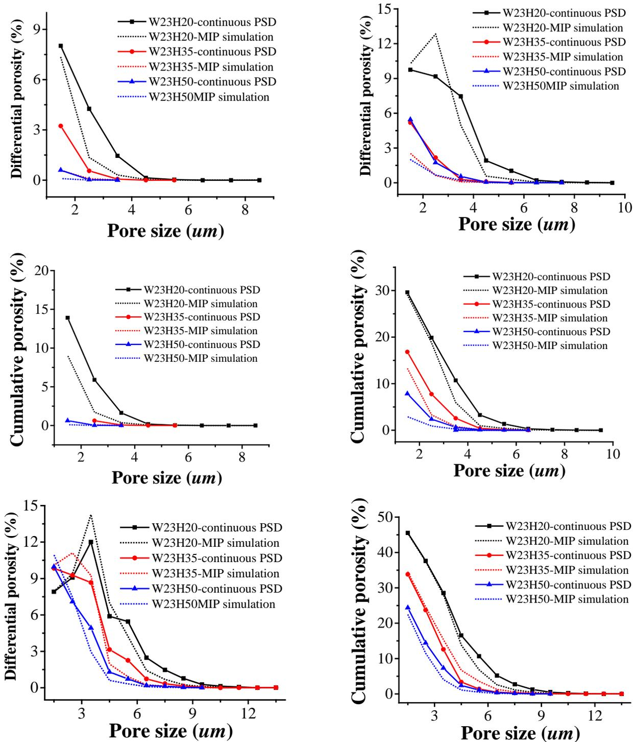
**Fig. 5.** The pore size distribution in each microstructure by MIP Simulation, and the algorithm of “Continuous PSD” (W23H35 represents the water cement ratio is 0.23 and hydration degree is 35%; MIP Simulation and Continuous PSD represent the results obtained by MIP Simulation, and the algorithm of “Continuous PSD”, respectively).
