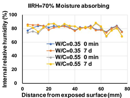
Fig. 14. Change in internal relative humidity in moisture absorbing process, IIRH=70%
