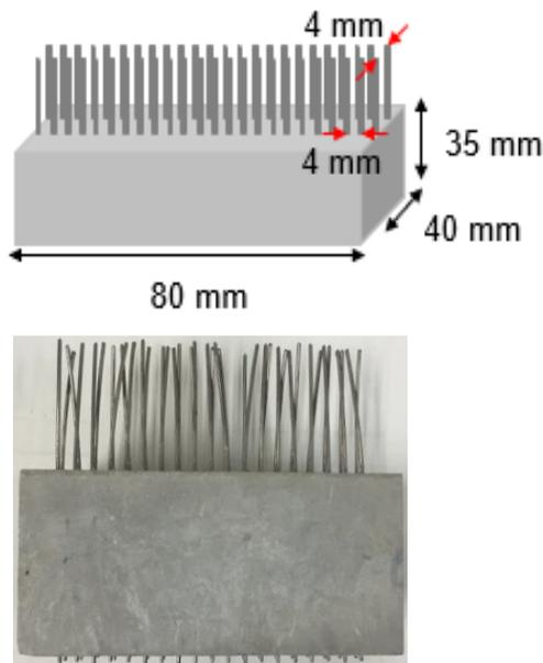
**Fig. 1.** Specimen configuration for moisture transfer test
