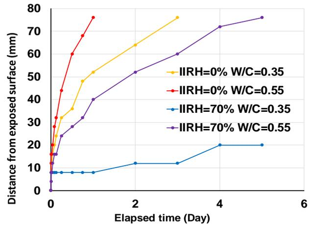
Fig. 9. Relationship between the distance of moisture transfer and elapsed time
