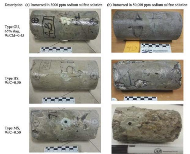
**Fig. 2.** Visual Condition of Concrete Cylinders after 38 Years Immersed in Sodium sulfate Solution: Left: in 3000 ppm  $\text{SO}_4$ ; Right: in 50,000 ppm  $\text{SO}_4$ . Note: Type GU cement had 12.3%  $\text{C}_3\text{A}$ ; Type MS cement had 7.1%  $\text{C}_3\text{A}$ ; Type HS cement had 3.5%  $\text{C}_3\text{A}$
