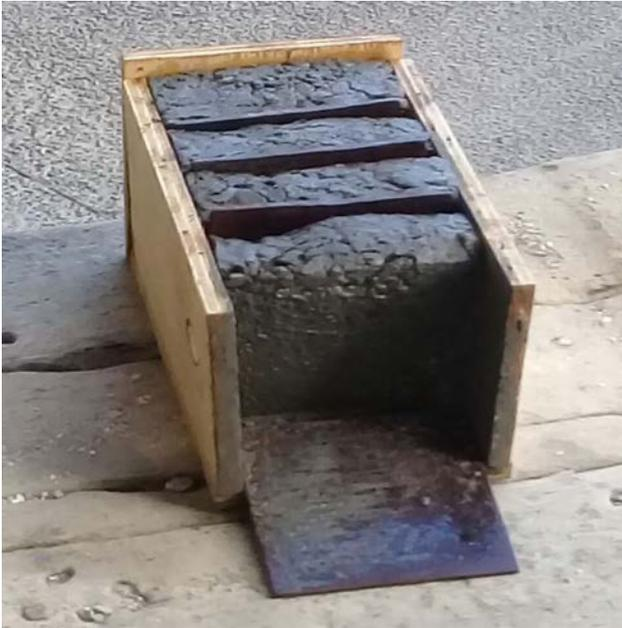
**Fig. 1.** Photo of method of slices apparatus with metal slides inserted
