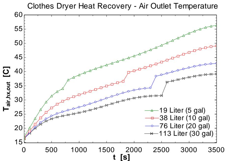
**Figure 3:** Cooled dryer exhaust air leaving the waste heat exchanger as a function of the storage tank volume
