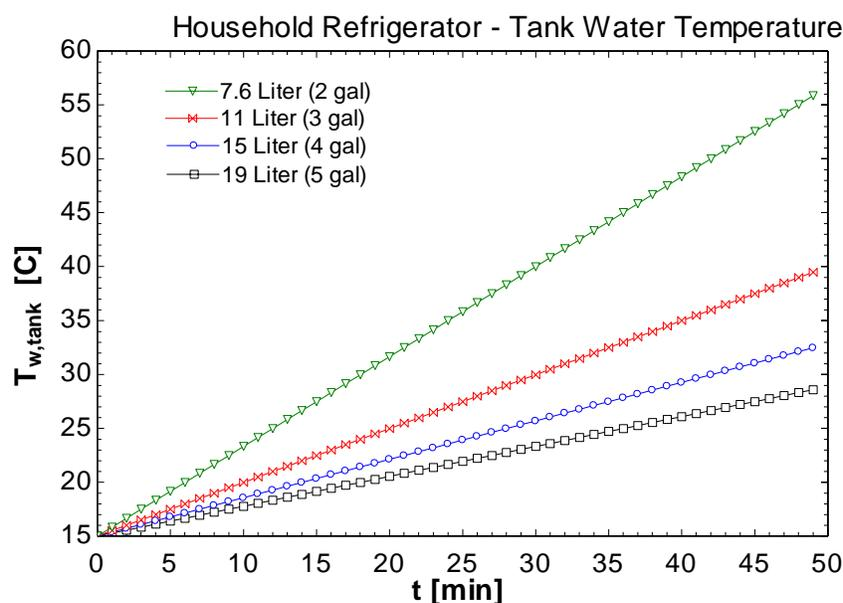
**Figure 1:** Storage tank temperature for water cooled condenser of household refrigerator
