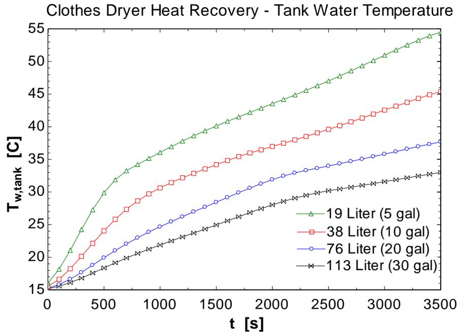
**Figure 2:** Impact of the storage tank volume size on the water temperature stored in the tank
