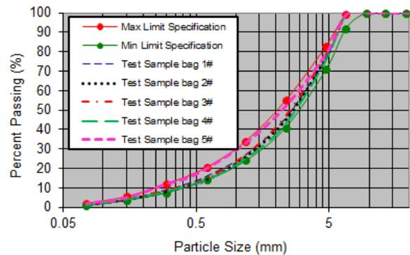
Fig. 2. Particle Size Distribution of Quartz sands
