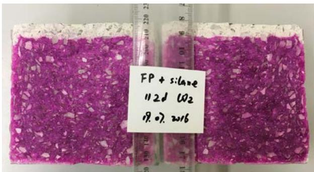
**Fig. 3.** Foreva MLC Form & Pour winter mix + Silane after 112 days CO<sub>2</sub> expose
