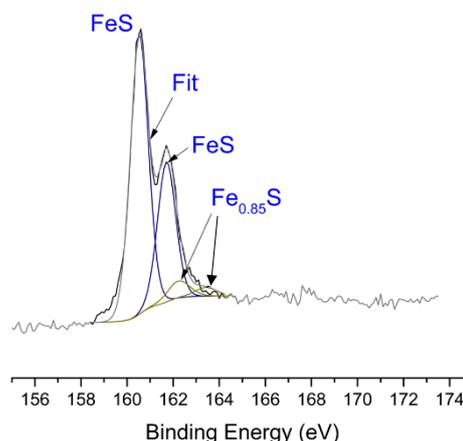
**Fig. 6.**  $\text{S}_{2p}$  XPS results for the passive film formed on steel after immersion in simulated alkali-activated slag pore solution (0.80 M NaOH + 0.45 M  $\text{Na}_2\text{S}$ )
