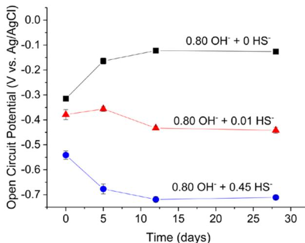
**Fig. 3.**  $E_{\text{corr}}$  values recorded for steel immersed in alkaline solutions ( $0.80 \text{ M OH}^-$ ) with varying concentrations of  $\text{HS}^-$  (0, 0.01 and 0.45 M)
