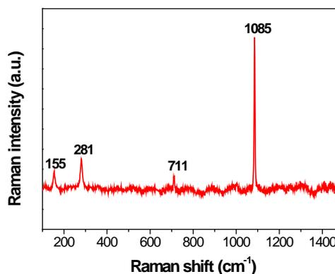
**Fig. 5.** Raman spectrum of the film detected on the steel surface shown in Fig. 4
