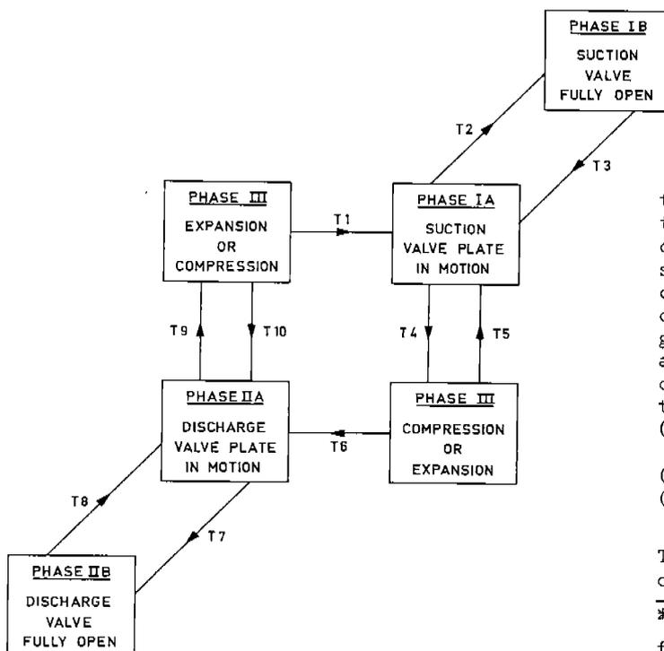
Fig. 4. Possible changes of one phase of operation into another. The symbols T1...T10 refer to conditional equations (not listed here).
