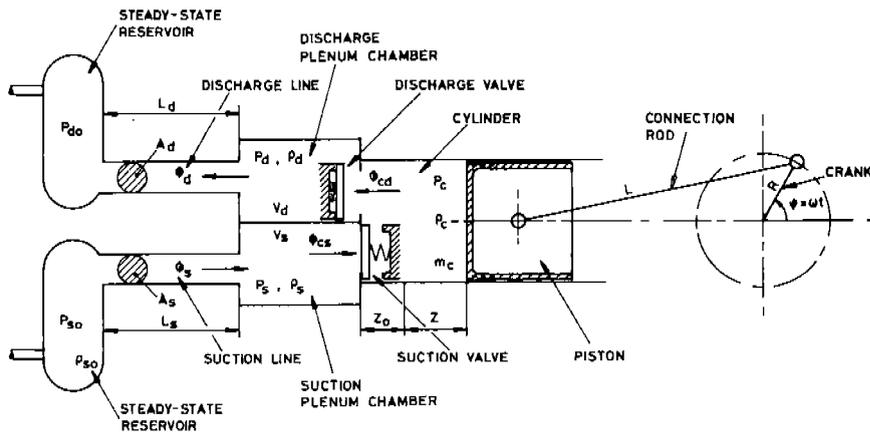
Fig. 1. Compressor model, showing the various system elements.
