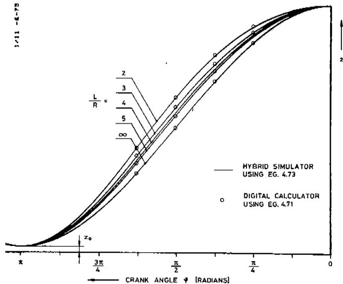
Fig. 3. Output of analog piston displacement generator, compared with some exact values of  $z$ .
