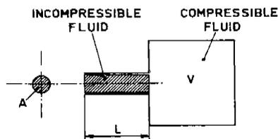
Fig. 2. Helmholtz resonator concept.
