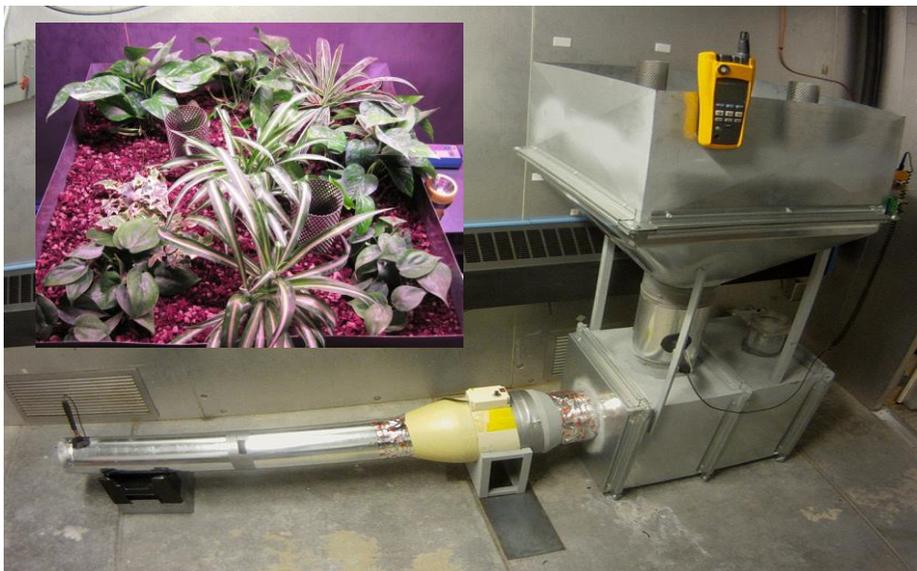
Figure 4. Biowall test apparatus in an environmental chamber.
