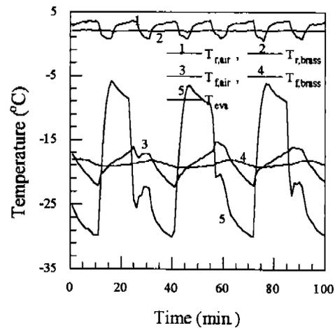
Fig. 4 Control characteristics of the new refrigerator
