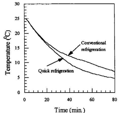
Fig. 7 Comparison of the refrigerating speed of 100 g water in the R-compartment
