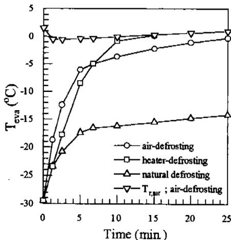
Fig. 8 Evaporator surface temperature during the defrosting cycle and air temperature in the R-compartment
