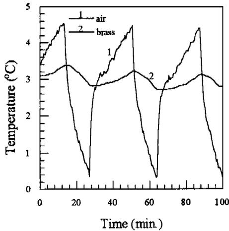
Fig. 5 Refrigerating compartment temperature, Conventional refrigerator
