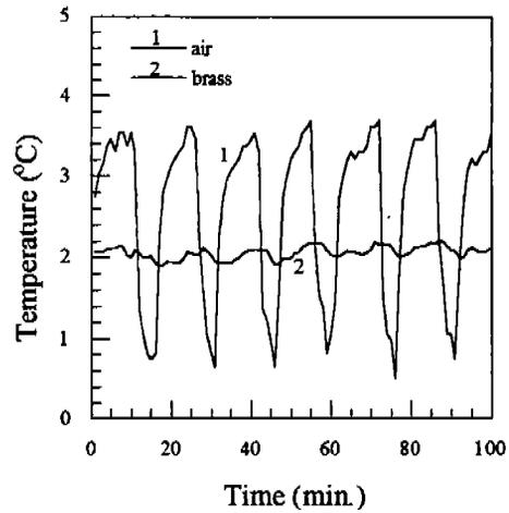
Fig. 6 Refrigerating compartment temperature, New refrigerator
