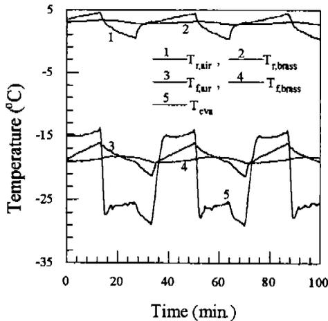
Fig. 3 Control characteristics of the conventional refrigerator
