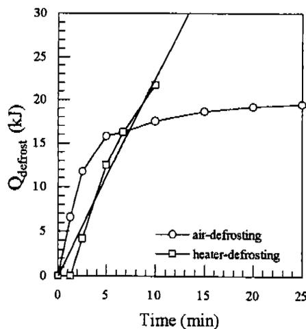
Fig. 9 Heat exchanged during the defrosting cycle ; air-defrosting and heater-defrosting
