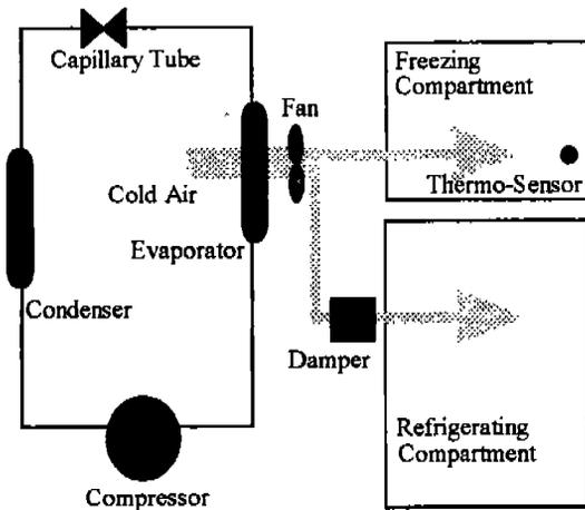
Fig. 1 Schematic of the conventional refrigerator with one cooling fan
