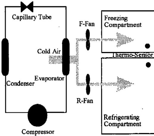
Fig. 2 Schematic of the new refrigerator with two cooling fans
