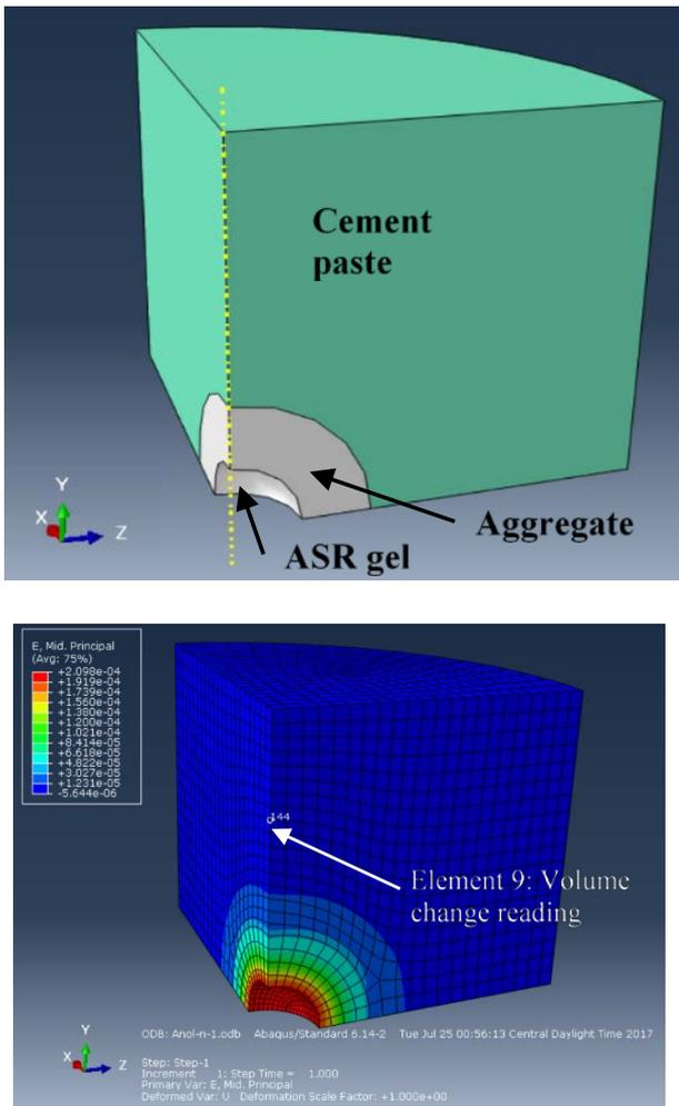
**Fig. 6.** RVE structure and strain distribution in FE
