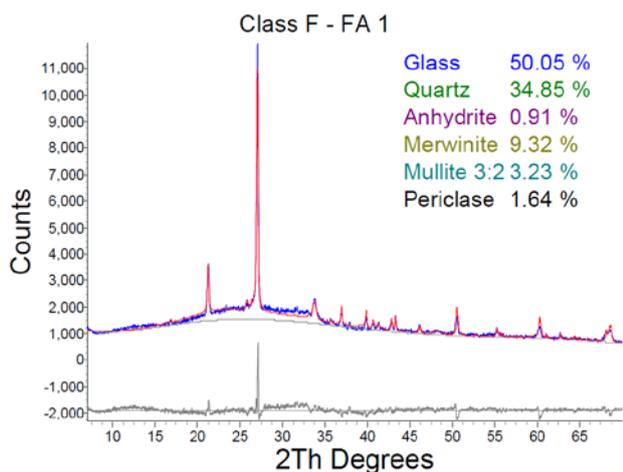
**Fig. 3.** XRD spectrum of FA type 1 used in this study
