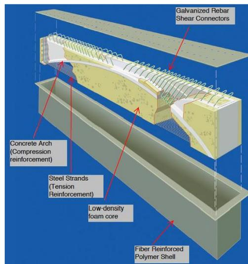
FIGURE 1 EXPLODED VIEW OF A TYPICAL HCB
