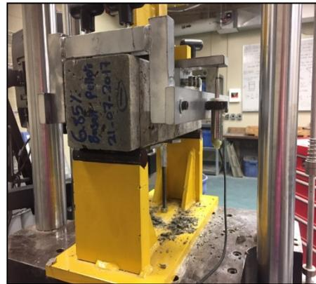
**Fig. 2.** Flexural test set-up
