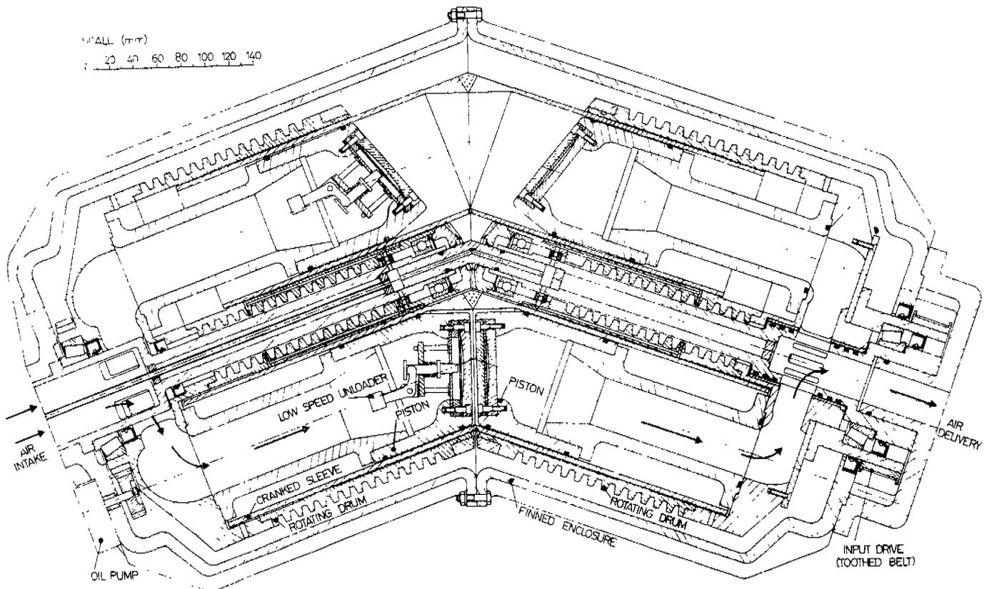
Fig.2 Shaw Type Rotary Compressor -  $40^\circ$  sleeve angle
