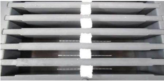
**Fig. 6a.** Central splitting of the test piece with the PE foam divider
