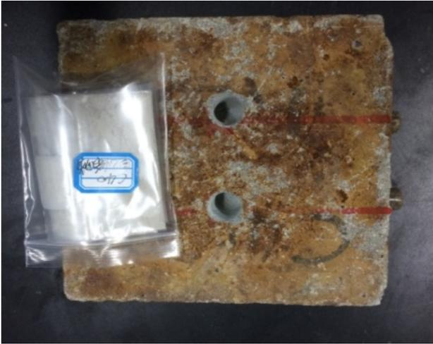
**Fig. 6.** Concrete block powder extraction
