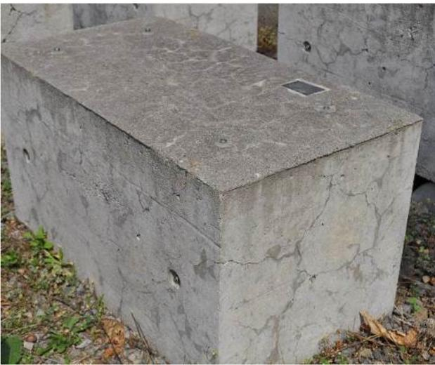
**Fig. 10.** Condition of exposure block NMLiOH1.0 after 15 years outdoors (0.390% expansion)
