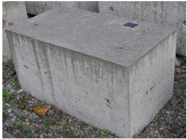
**Fig. 13.** Condition of exposure block NMLiN1.25 after 15 years outdoors (0.041% expansion)
