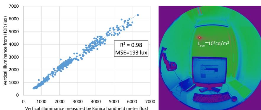
**Figure 2:** Validation of HDR imaging in terms of vertical illuminance (left); HDR image indicating the luminance of the sun after application of filter and calibration (right)
