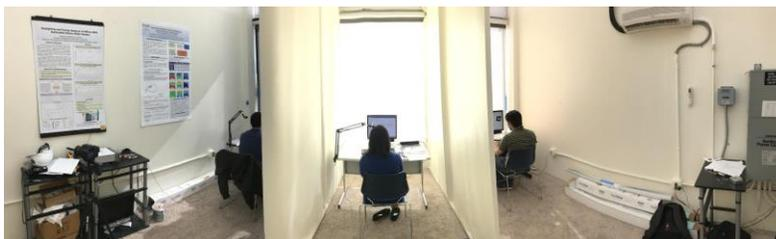
**Figure 1:** Experimental layout of one of the two identical offices used for the study with three partitioned workstations, each equipped with a different shade.
