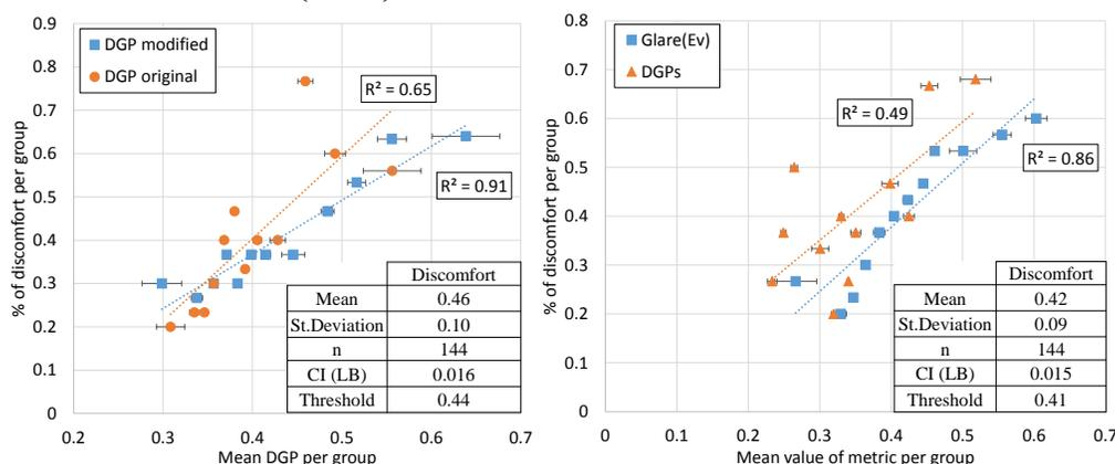
**Figure 7:** Improvement of fit for the modified DGP compared to original (left) and for the new illuminance-based metric compared to DGPs (right)
