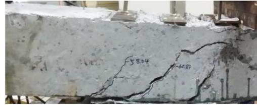
Fig.5. Combined failure of L1500-150-2.
