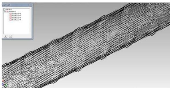
Fig.1. Point cloud of reinforcing bar from scanning
