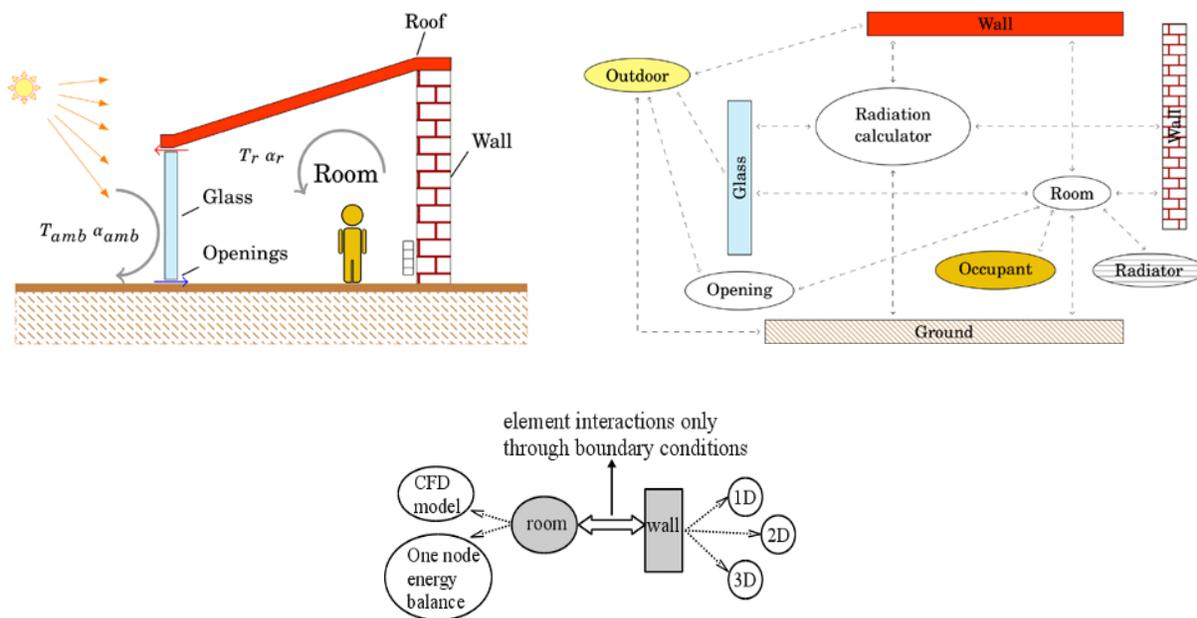
**Figure 1.** (top-left) Scheme of a room. (top-right) NEST views the system as a vertex-edge graph. (bottom) Flexibility in choosing individual elements models.
