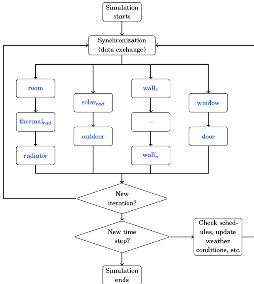
**Figure 2.** Block-Jacobi like algorithm implemented in NEST-Buildings.
