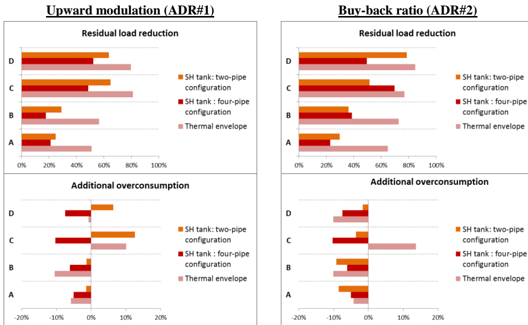
Figure 6: Comparison of ADR#1 and ADR#2 for houses A to D and three storage options. Average values over two winter days and one day in the spring.
