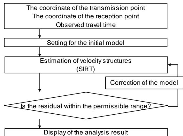
**Fig. 4.** Procedure of the ultrasonic tomography analysis
