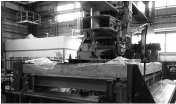
**Fig. 2.** Wheel running test machine
