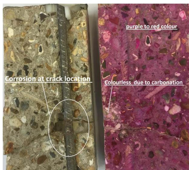
**Fig.10.** Corrosion of reinforcement bar at the location of a crack due to exposing to CO<sub>2</sub> with 65% of RH
