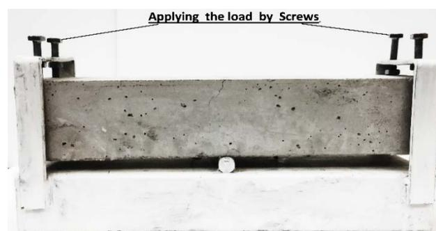
**Fig. 1.** Flexural method was used to create the crack in concrete sample
