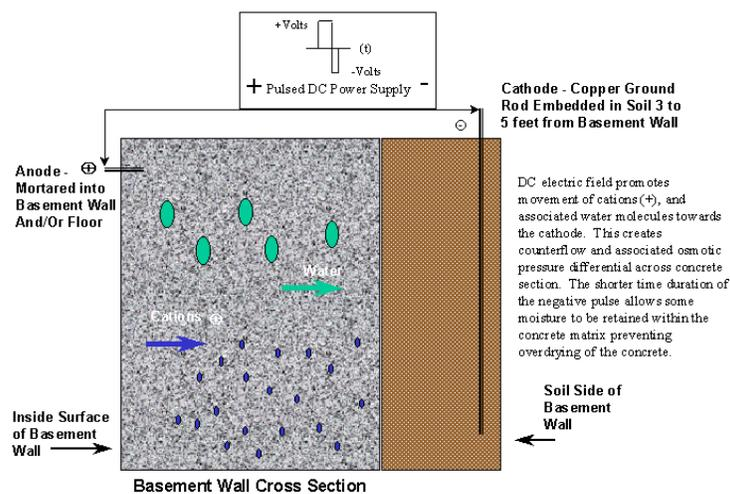
FIGURE 3 ELECTRO OSMOTIC PULSE TECHNOLOGY FOR PREVENTION OF WATER INTRUSION IN CONCRETE BASEMENTS
