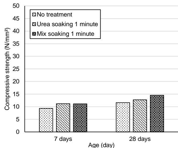
**Fig. 4.** Compressive strength test results when immersed in an aqueous solution (W/C=60 %)
