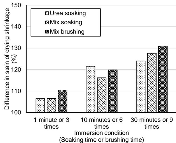
**Fig. 10.** The comparison of length change rates when soaking for 1 minute, 10 minutes, 30 minutes and brushing for 3, 6, 9 times (W/C=50 %)
