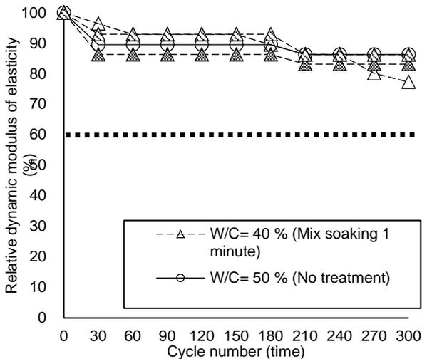
**Fig. 16.** The results of the freeze-thaw test
