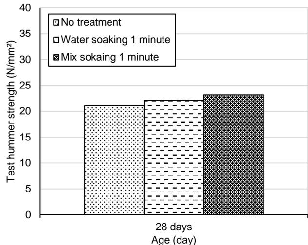
**Fig. 18.** The results of the test hammer strength test
