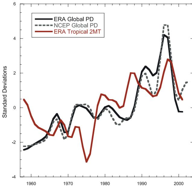
**Figure 2.** ERA-40-derived global PD (black curve), NCEP-derived global PD (dashed curve) and ERA-40 mean annual tropical 2MT (red curve). Tropical 2MT is averaged annually from 30 degrees north to 30 degrees south globally, and all curves are normalized with the respective standard deviations of the detrended time series. The correlation between ERA-40 PD and ERA-40 2MT is  $r^2 = 0.34$ .
