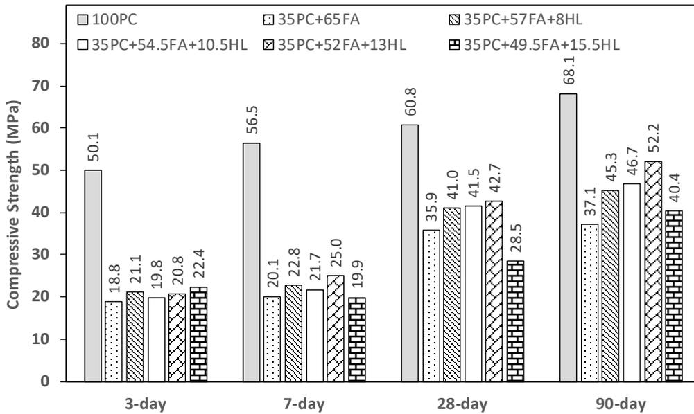
Fig. 1. The compressive strength development of HVFA-65 concrete
