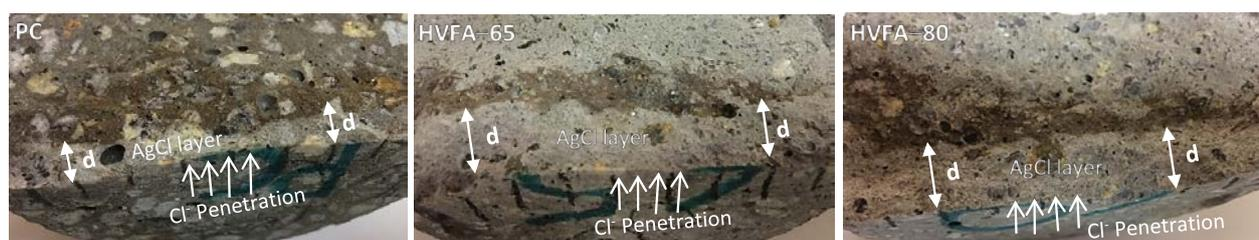
**Fig. 3.** Chloride penetration depth in different concretes
