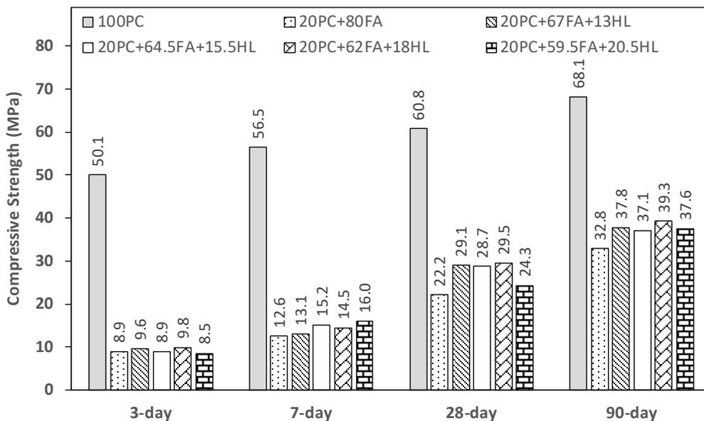
Fig. 2. The compressive strength development of HVFA-80 concrete
