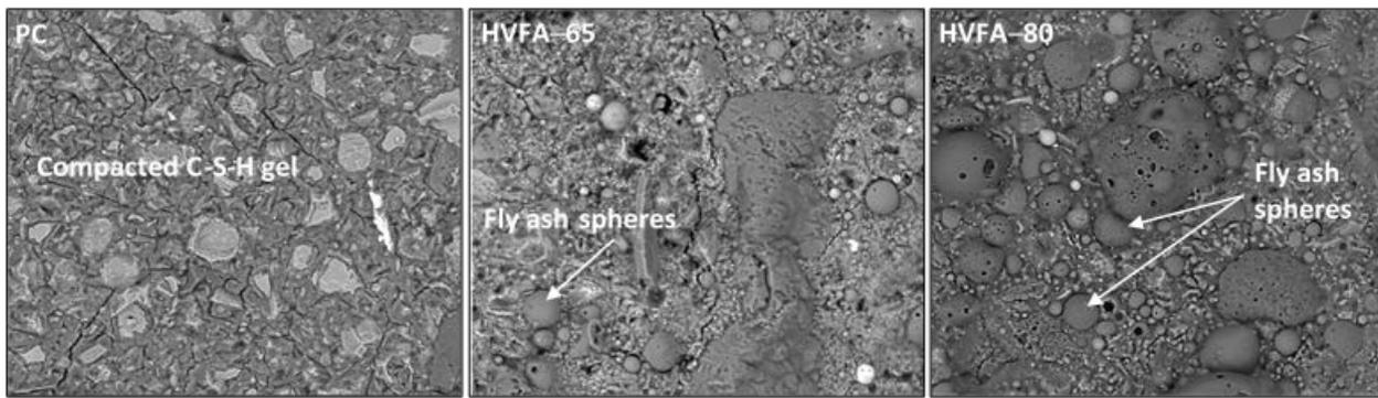
**Fig. 5.** Microstructure variation of PC and HVFA concretes at 28 days
