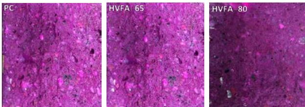
**Fig. 4.** Carbonation depth in different concretes
