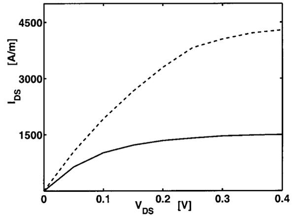
FIG. 9. Ballistically simulated (non-self-consistent, potential profiles obtained from self-consistent scattering simulations are used)  $I-V$  characteristics for the UN (dashed line) and WN (solid line) devices indicate that the on-currents for the two device structures could differ by as much as  $\sim 250\%$ . In contrast, once scattering is included, the  $I-V$  characteristics for the two devices differ by no more than  $\sim 10\%$ .
