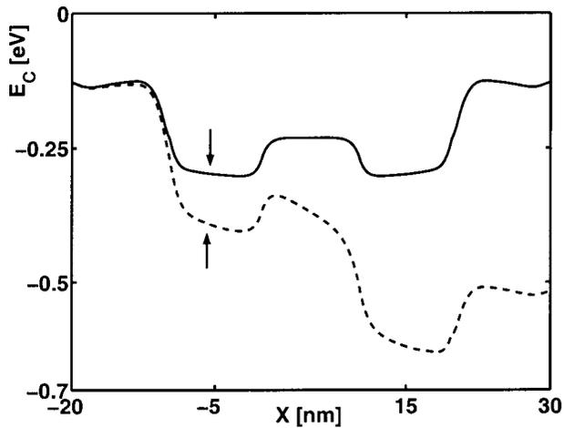
FIG. 10. Averaged conduction band profile within the WN device (on-state) at equilibrium (solid line) and on the application of a large drain voltage (dashed line,  $V_{DS}=0.4$  V). It is clear that the conduction band edge is unchanged within the large S/D reservoirs as they maintain a near-equilibrium distribution even when a large drain bias is applied. The conduction band within the intrinsic source [Fig. 1(b)] floats to lower values to enforce charge neutrality [Fig. 6(b)].
