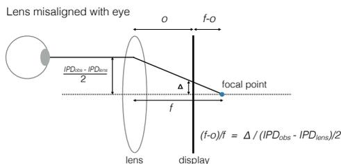
**Fig. 1:** When the lens and display are misaligned with the eye, the vergence angle of each eye changes to compensate for the lateral shift,  $\Delta$ , between the display center (equivalent to optical axis) and where the refracted line of sight, due to the prismatic effect, intersects the display. The principle of similar triangles can be used to solve for  $\Delta$ , given the expression on the right.
