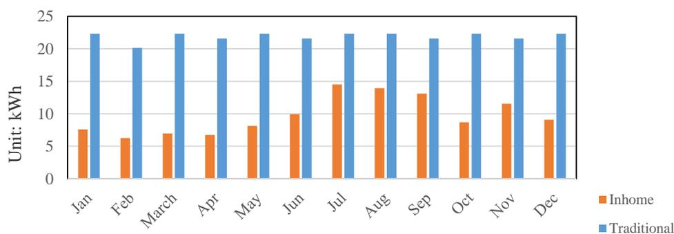
**Figure 7.** Monthly energy consumption of ERV system.
