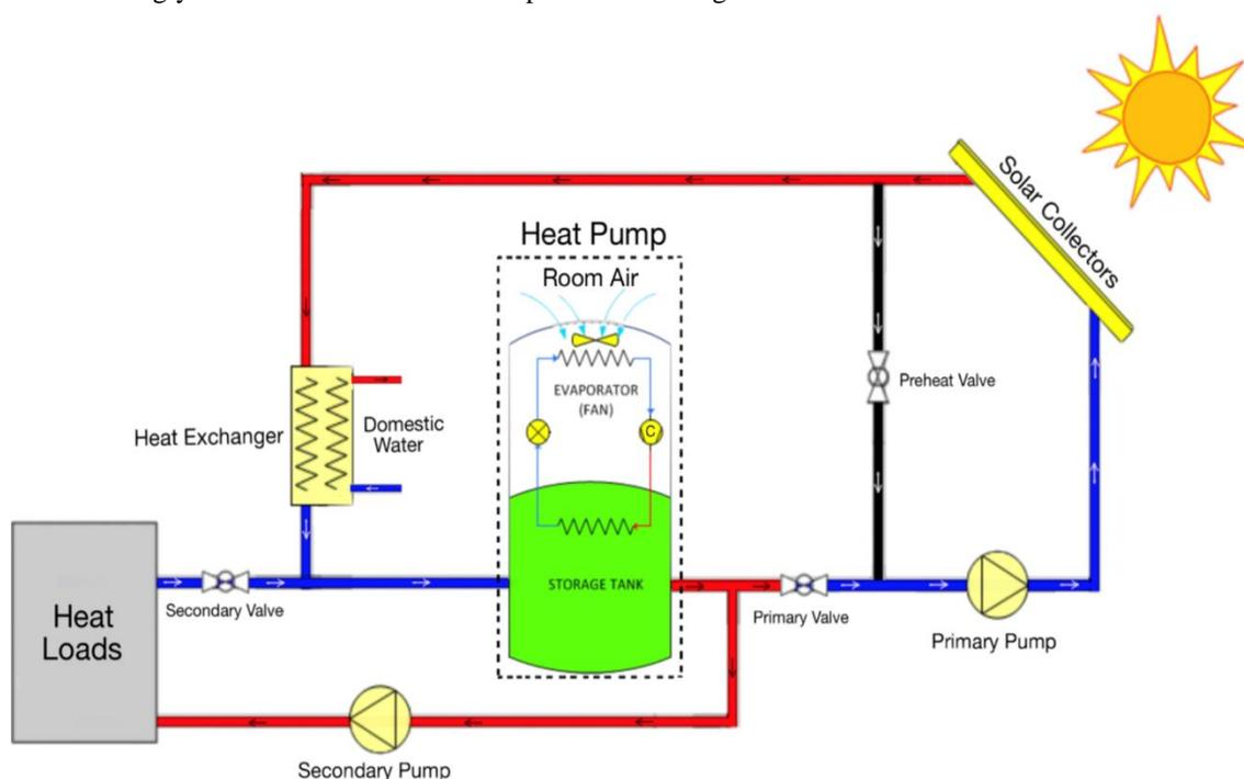
**Figure 1:** The SHPS has primary and secondary loops.
