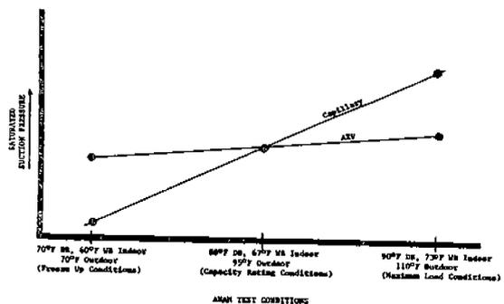
Through the use of system balance charts, additional benefits of employing constant pressure expansion valves on air conditioning systems can be demonstrated. These additional benefits include: improved capacity and operating efficiency through more efficient compressor operation and increased evaporator loading; and reduced first cost through
