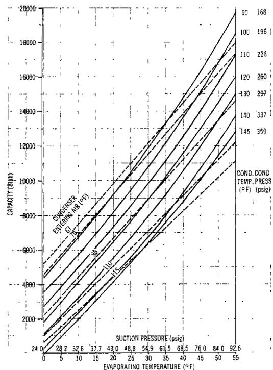
Figure 4 presents the same compressor-condenser curves with the addition of evaporator capacity performance curves for a typical evaporator using a capillary tube. Evaporator performance is plotted at constant evaporator entering air conditions. Figure 4 is a complete system balance with all three major system components represented. At AHAM rating conditions of 80° DB, 67° WB evaporator entering air temperature, and 95° condenser entering air, one will note that the system
