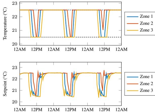
Figure 5: Low-Level Airside Optimization Result.
