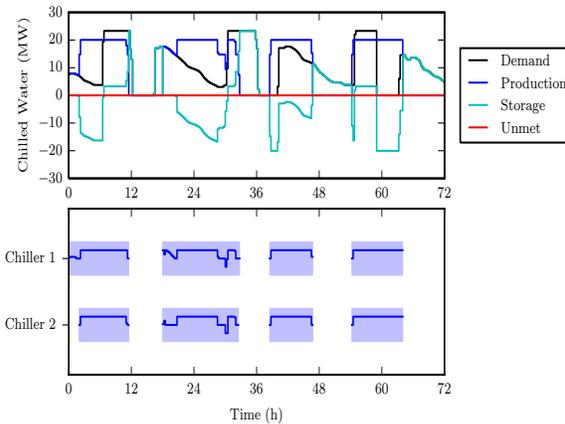
Figure 6: Low-Level Waterside Optimization Result.
