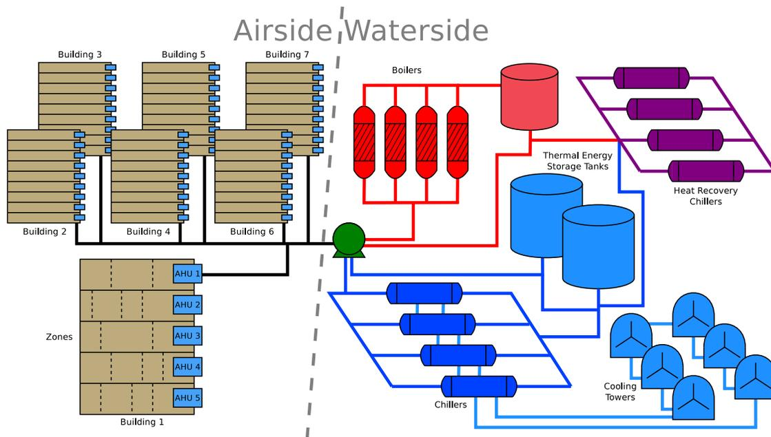
**Figure 1: Schematic of large-scale commercial application with airside system shown on the left and waterside system shown on the right.**
