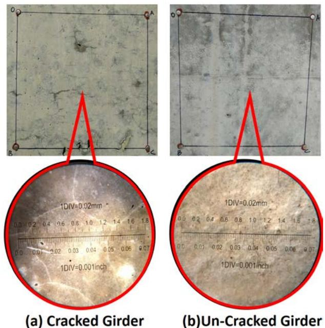
**Fig. 6.** Typical regions on an (a) extensively cracked and (b) un-cracked girder as visible to the naked eye (top row of photos) and at 50X magnification (shown in the circled call-out)
