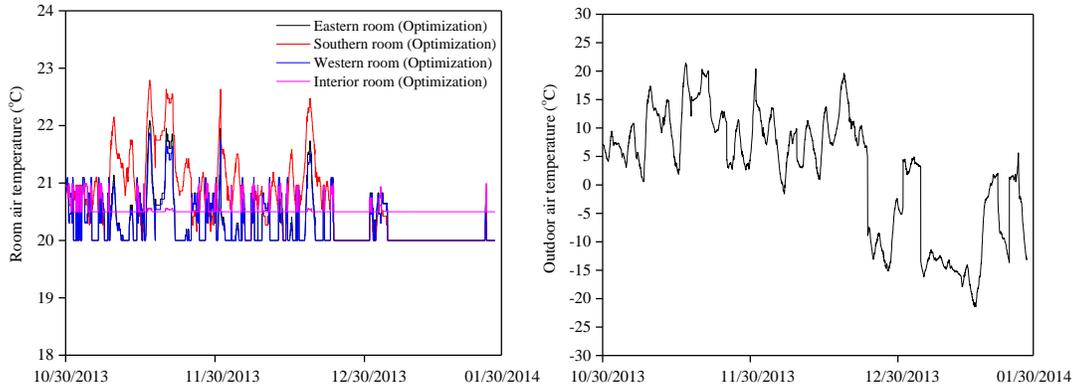
**Figure 4:** Room air temperatures from the case with optimal control and outdoor air temperature
