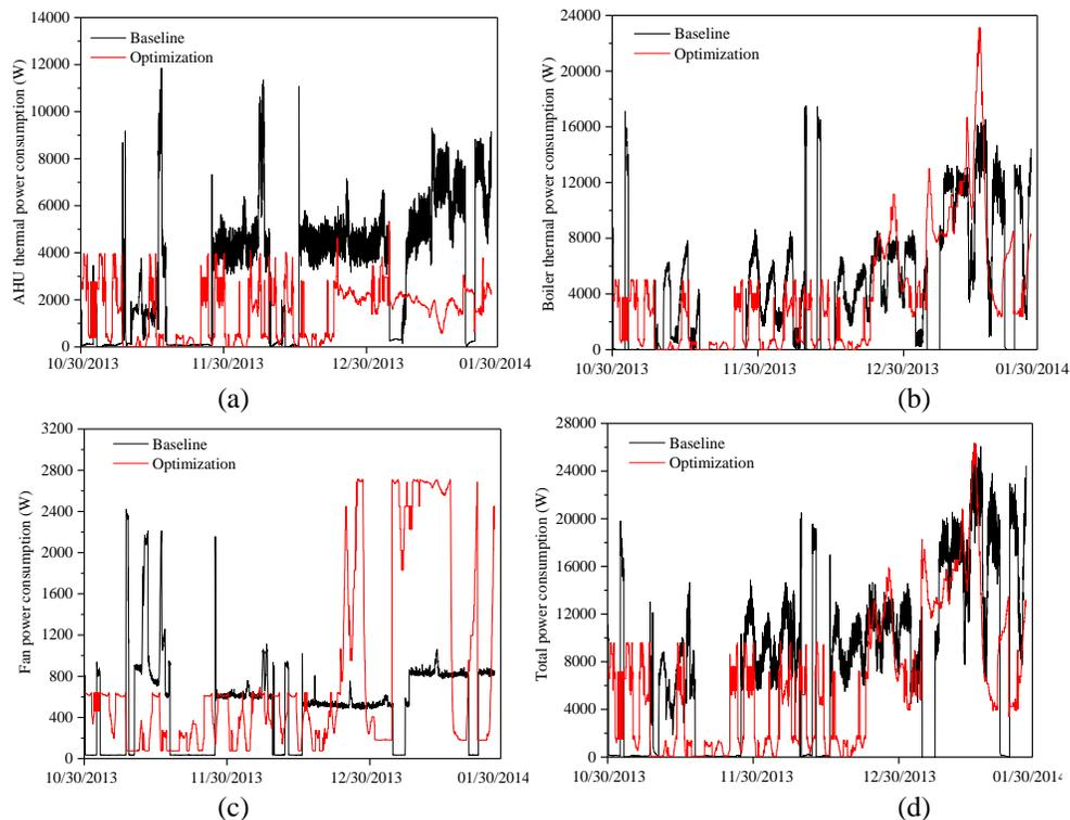
**Figure 8:** (a) AHU thermal power consumption; (b) VAV box reheat thermal power consumption; (c) Fan power consumption; (d) HVAC system total power consumption
