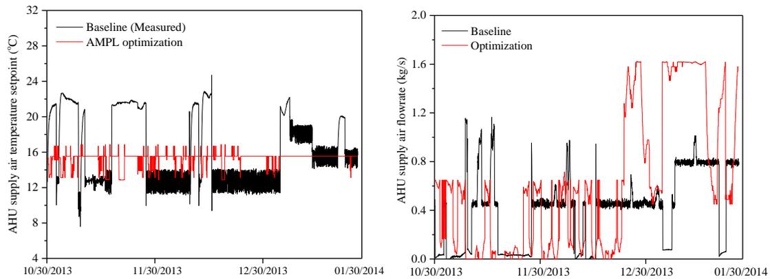
**Figure 5:** Optimized AHU supply air temperature and air flowrate
