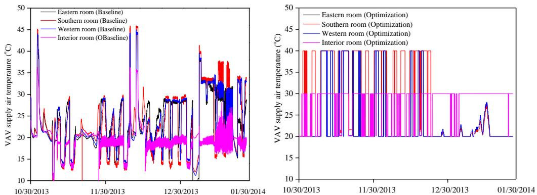
**Figure 6:** VAV box supply air temperature
