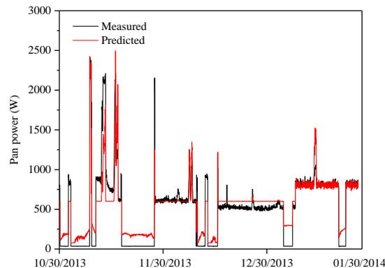
**Figure 2:** Fan electrical power consumption comparison
