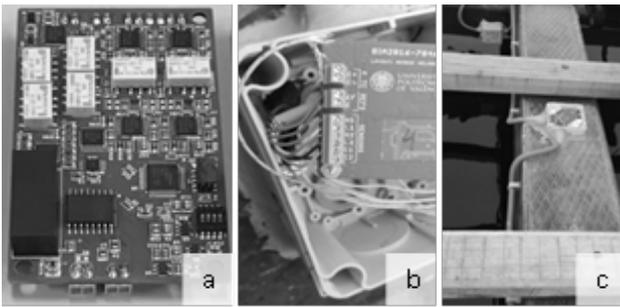
**Fig. 4.** a) Printed circuit board with an integrated miniaturized potentiostat; b) and c) Circuit board installed as a measurement node at one of the control points (CP) inside a specific waterproof box.
