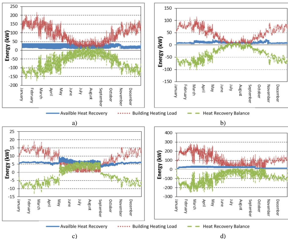
**Figure 6:** Required heat recovery and availability heat recovery for a) XR-02 b) XR-03/14 c) XR-04 d) XR-12/15
