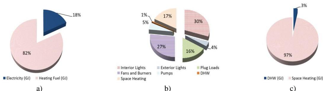
**Figure 3:** Distribution of a) Energy for the PCSP facility b) Electricity consumption by end-use c) Fuel use
