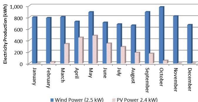
**Figure 5:** Monthly comparison of electricity production between a 2.5 kW wind turbine and a 2.4 kW PV array
