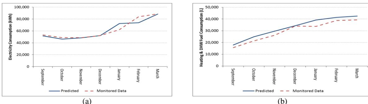
**Figure 2:** Comparison of simulated and recorded (a) electricity and (b) fuel consumption for the 2015/2016 FY
