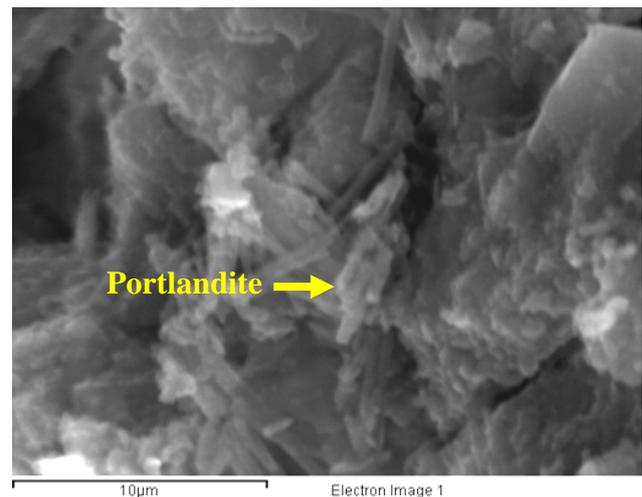
Fig. 3. SEM image of CC concrete (x 5000)
