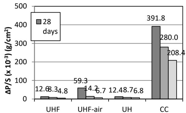
Fig. 6. Water absorption by capillarity per unit area
