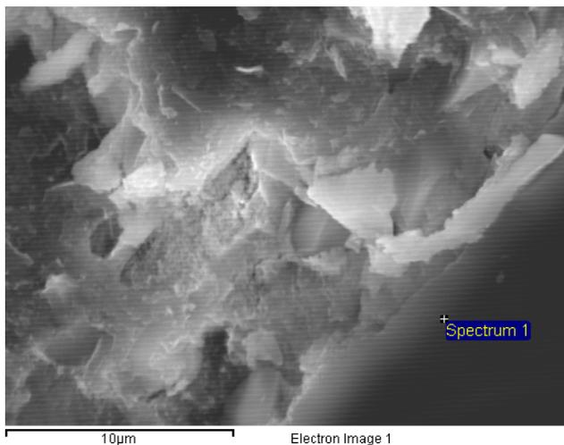
Fig. 1. SEM image of UH concrete (x 5000)
