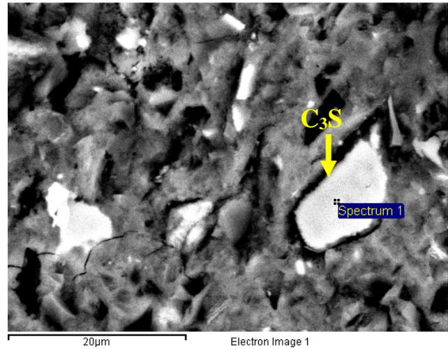
Fig. 2. Backscattered electron (BSE) image of UH concrete
