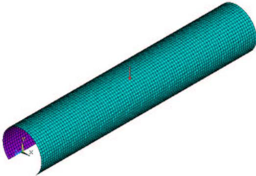
**Fig. 2** Full, 3-D finite element model of incomplete, orthotropic circular cylindrical shell implanted in ANSYS version 5.7. Arrow at the center indicates point input force.
