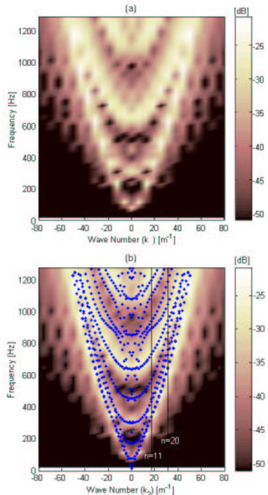
**Fig. 3** (a) Frequency-wave number domain representation of the forced responses obtained from full, 3-D FE analysis and (b) dispersion relations (dots) obtained from hybrid 2-D FE analysis overlaid on forced responses (contour) presented in Fig 3(a).
