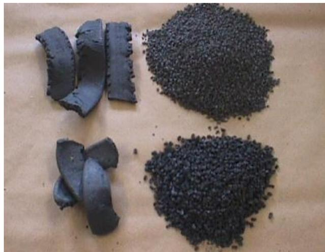
**FIGURE 2 EXTRUDATES BEFORE AND AFTER GRANULATION (COURTESY OF GEI CONSULTANTS INC.)**
